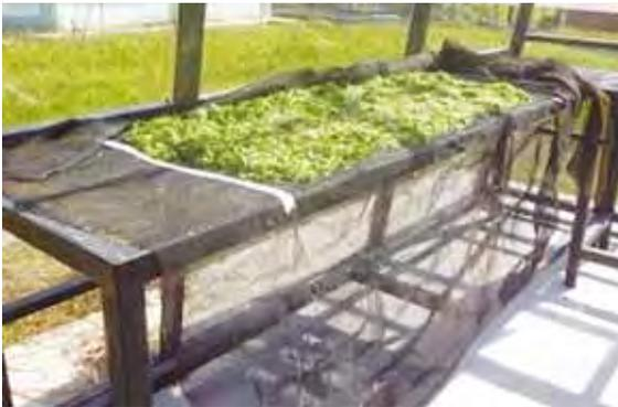
**Figure 5:** Drying bed without heater and blower of the greenhouse solar dryer
