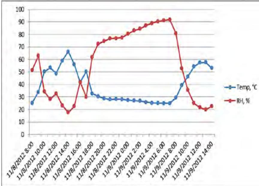
**Figure 7:** Temperature and relative humidity inside the drying chamber of the greenhouse solar dryer
