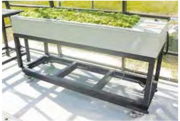
**Figure 4:** Drying bed with heater and blower of the greenhouse solar dryer
