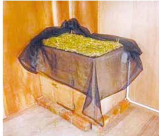
**Figure 2:** Drying bed of the prototype solar dryer
