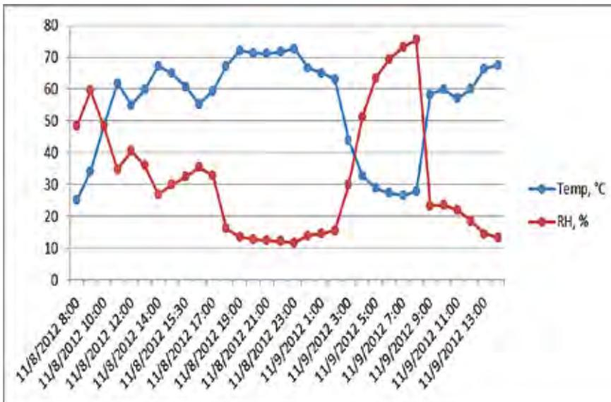
**Figure 8:** Temperature and relative humidity inside the drying bed of the greenhouse solar dryer
