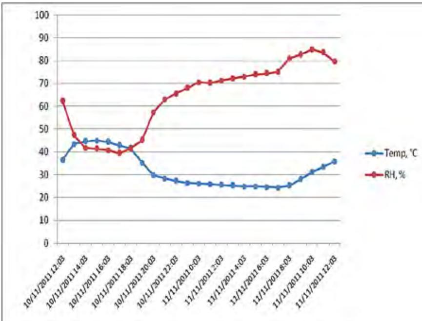
**Figure 6:** Temperature and relative humidity inside the drying bed of the prototype solar dryer
