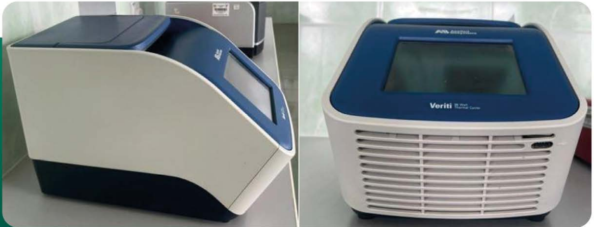
Rajah 1: Mesin Thermal Cycler PCR
